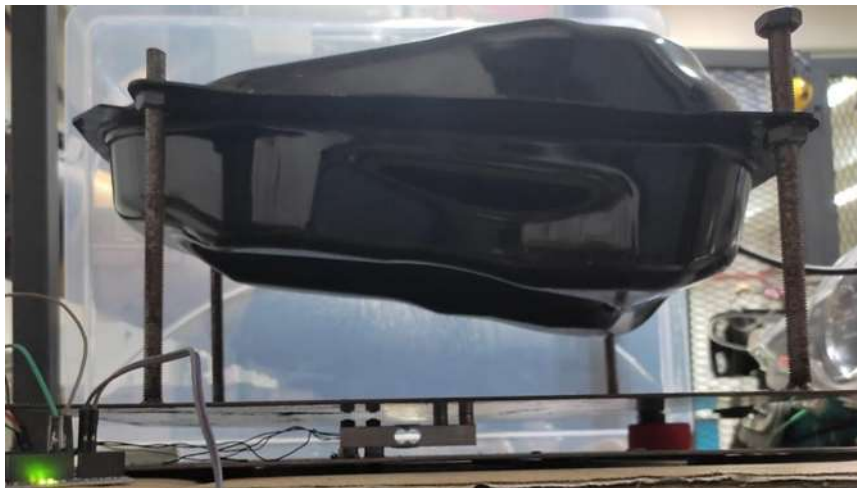
Figure 2: Electronic fuel weight scale setup
