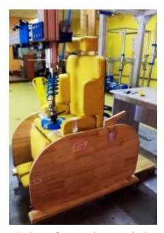
Figure 5: Seat front edge static load test
