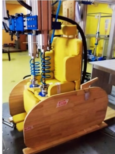
Figure 6: Seat front edge static load test
