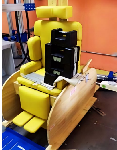
Figure 4: Sideways overbalancing test
