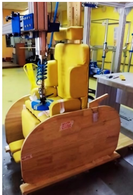
Figure 5: Seat front edge static load test
