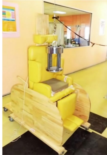
Figure 2: Seat impact test
