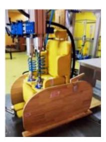
Figure 6: Seat front edge static load test
