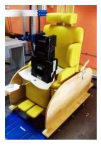
Figure 3: Forward overbalancing test
