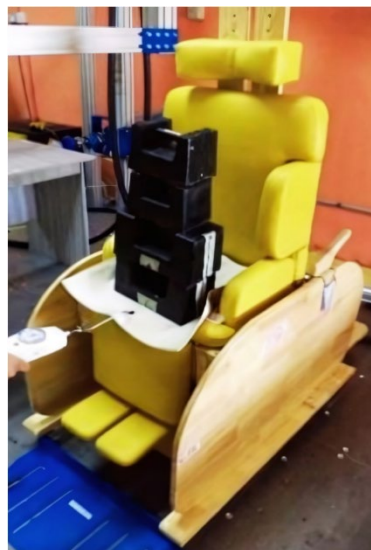
Figure 3: Forward overbalancing test
