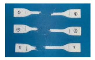
Figure 8: Tensile strength testing of 5% rWCO
