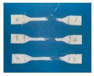
Figure 10: Tensile strength testing of 10% rWCO
