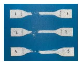
Figure 9: Tensile strength testing of 7.5% rWCO
