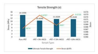
Figure 11: Tensile strength and strain at ultimate tensile strength (σ) graph
