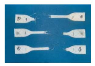
Figure 7: Tensile strength testing of 0% rWCO
