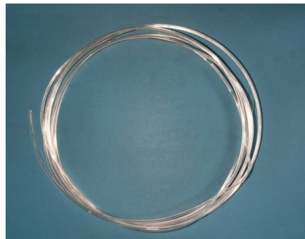
Figure 3: Filament produced from the extrusion process
