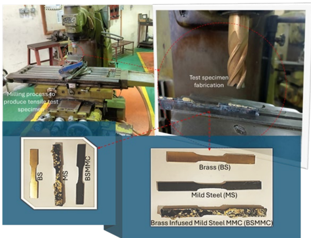
Figure 2: Tensile test specimen fabrication using a vertical milling machine
