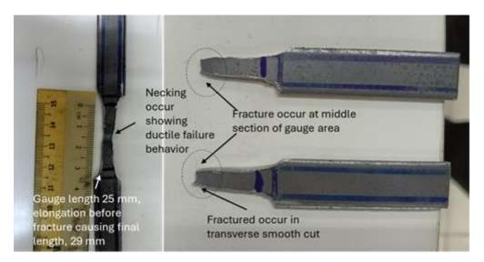
Figure 6: Failure modes of the mild steel test specimen
