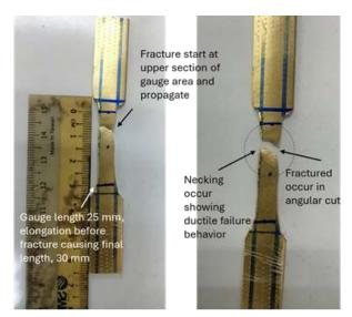
Figure 7:Failure modes of brass test specimen
