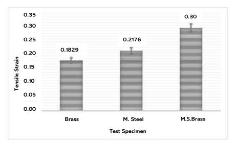
Figure 5: Tensile strain comparison among all test specimens
