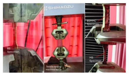
Figure 3: Mechanical test set-up
