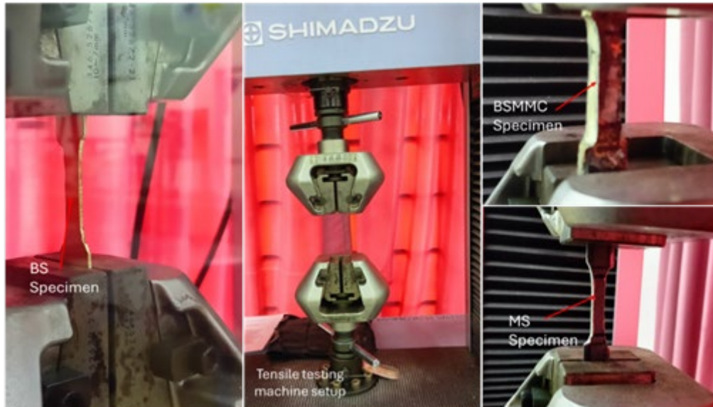
Figure 3: Mechanical test set-up
