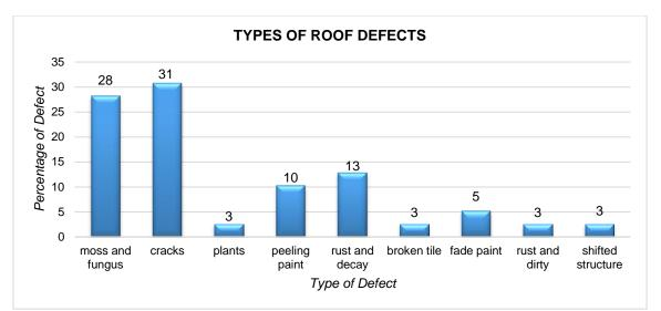
Figure 7: Graph of total roof defects according to defect types
