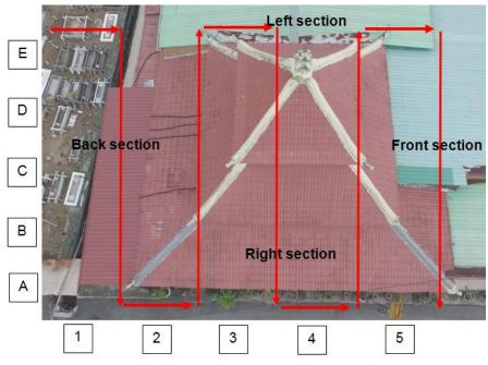
Figure 2: Flight direction according to roof section
