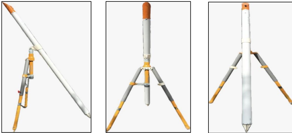
Figure 4: Fixed Pole-Jurin Design from Side, Front and Rear View consisting of Main Spike, Retainer Legs and Observation Mark with Plumb-Bob
