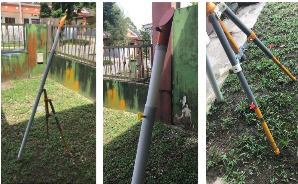
Figure 3: Fixed Pole-Jurin Made of Wasted Materials
