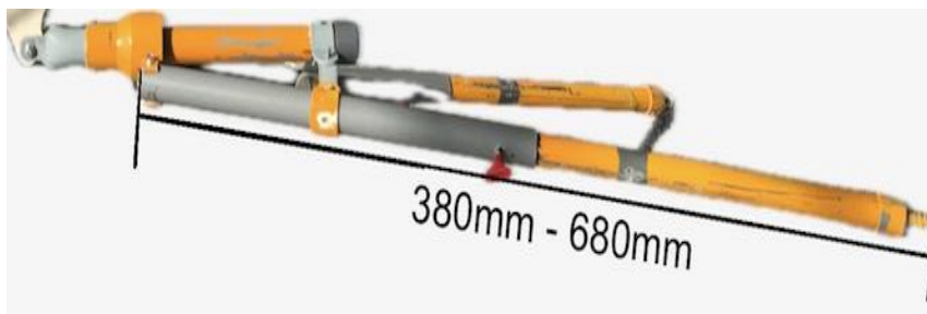
Figure 6: Supporting Leg with Dimensions Showing the Size of Openings
