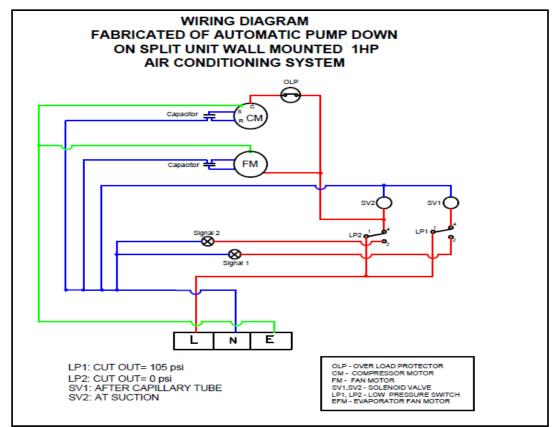
**Figure 3:** Wiring diagram fabricated of automatic pump down on split unit wall mounted 1hp air conditioning system
