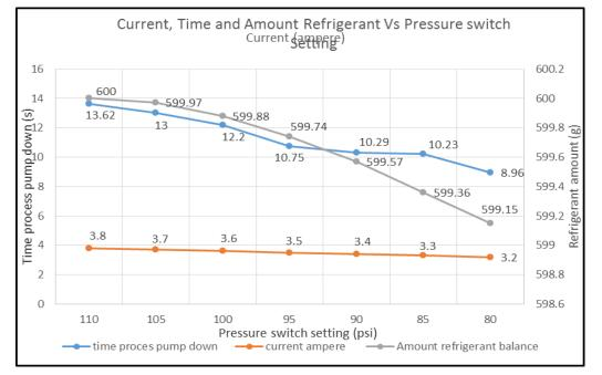
Figure 4: Current, time, and amount of refrigerant against the pressure switch setting
