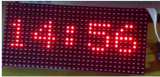
Figure 11: LED dot matrix display with timer; minute and second.
