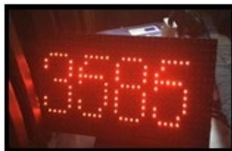
Figure 10: LED dot matrix display with number input.
