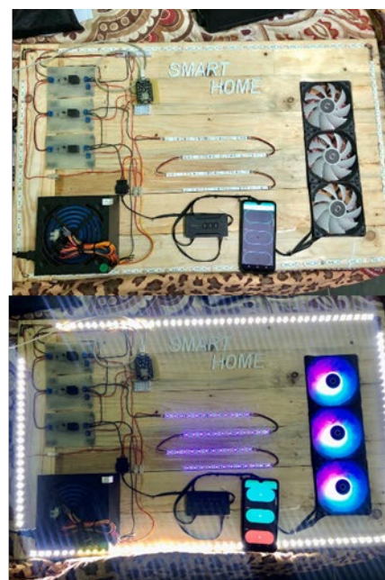
Figure 13: The prototype of Smart House Control System using Node MCU.
