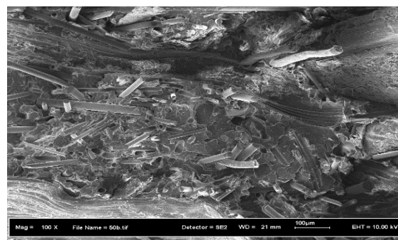
Figure 15: Magnification at mixture of 50 wt. % PP, 25 wt. %EG and 25 wt. 10% TB
