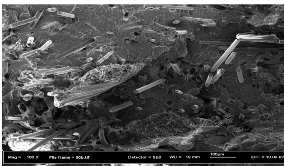
Figure 14: Magnification at mixture of 80 wt. % PP, 10 wt. %EG and 10 wt. 10% TB
