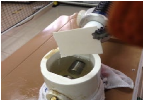
(a) Specimen inserted into test cell
