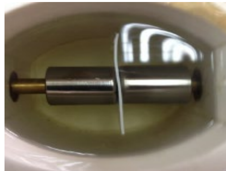
(b) Specimen and electrodes completely immersed with mineral oil
