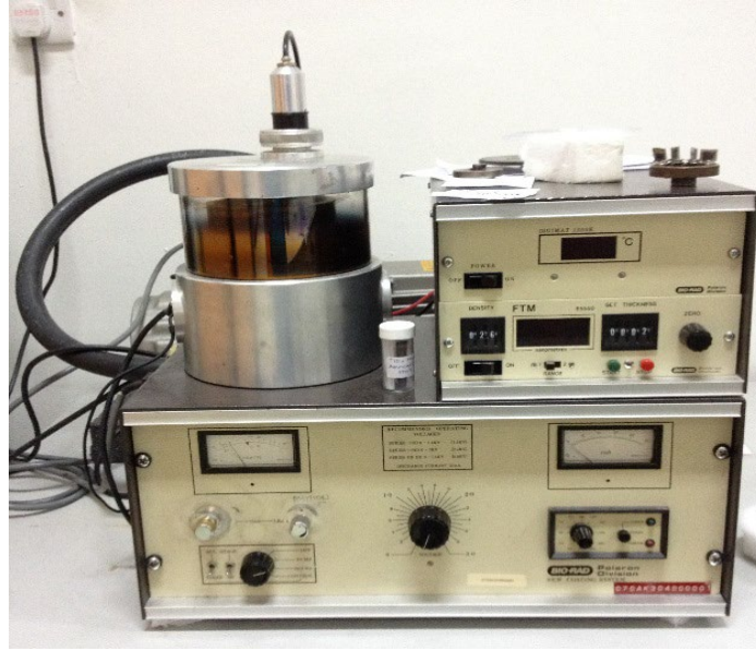
(a) Sputter coater model Polaron SC 515
