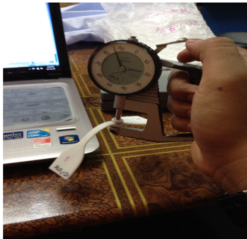
(a) Thickness gauge measurement
