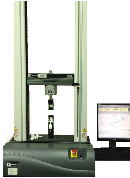
Figure 7: Instron 3360 universal testing machine (UTM)
