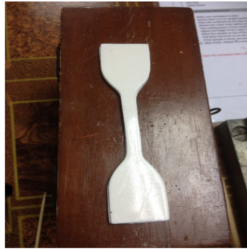
(b) Dumbbell specimen after cutting
