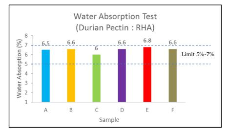
Figure 1: Result of water absorption test (ratio of durian pection: RHA)
