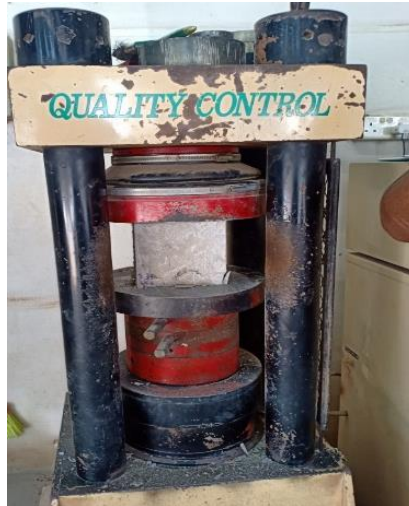
Figure 7: Compressive strength test
