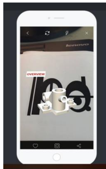
Figure 8: ARC-3DM augmented phase of second QR code displaying interactively 3D model reference in three dimensional view
