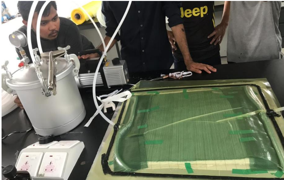
Figure 2: Vacuum infusion setup for fabrication of plate specimen
