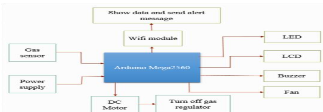
Rajah 2.2: Rajah blok LPG leakage detector system using arduino and internet of things (IoT)
