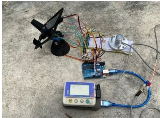
Figure 1: Complete setup with solar panel and pyranometer
