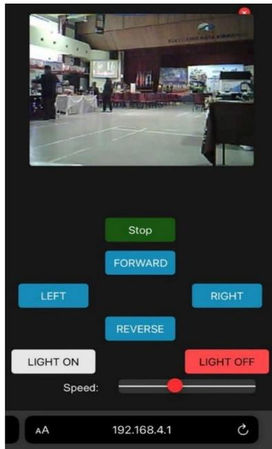
Figure 3: User interface platform for controlling the robot
