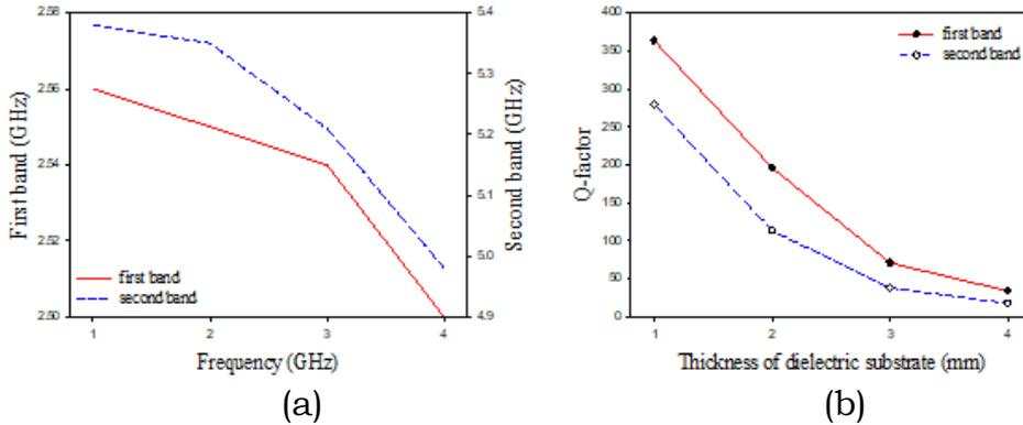
Figure 6: Dual band metamaterial absorber: (a) resonance frequencies for each band and (b) Q-factor according to the dielectric thickness
