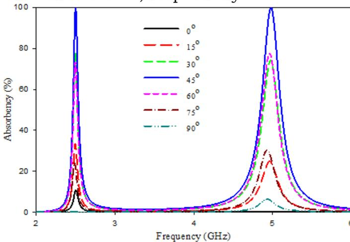
Figure 3: The absorption spectra of dual band metamaterial absorber at different rotation angle
