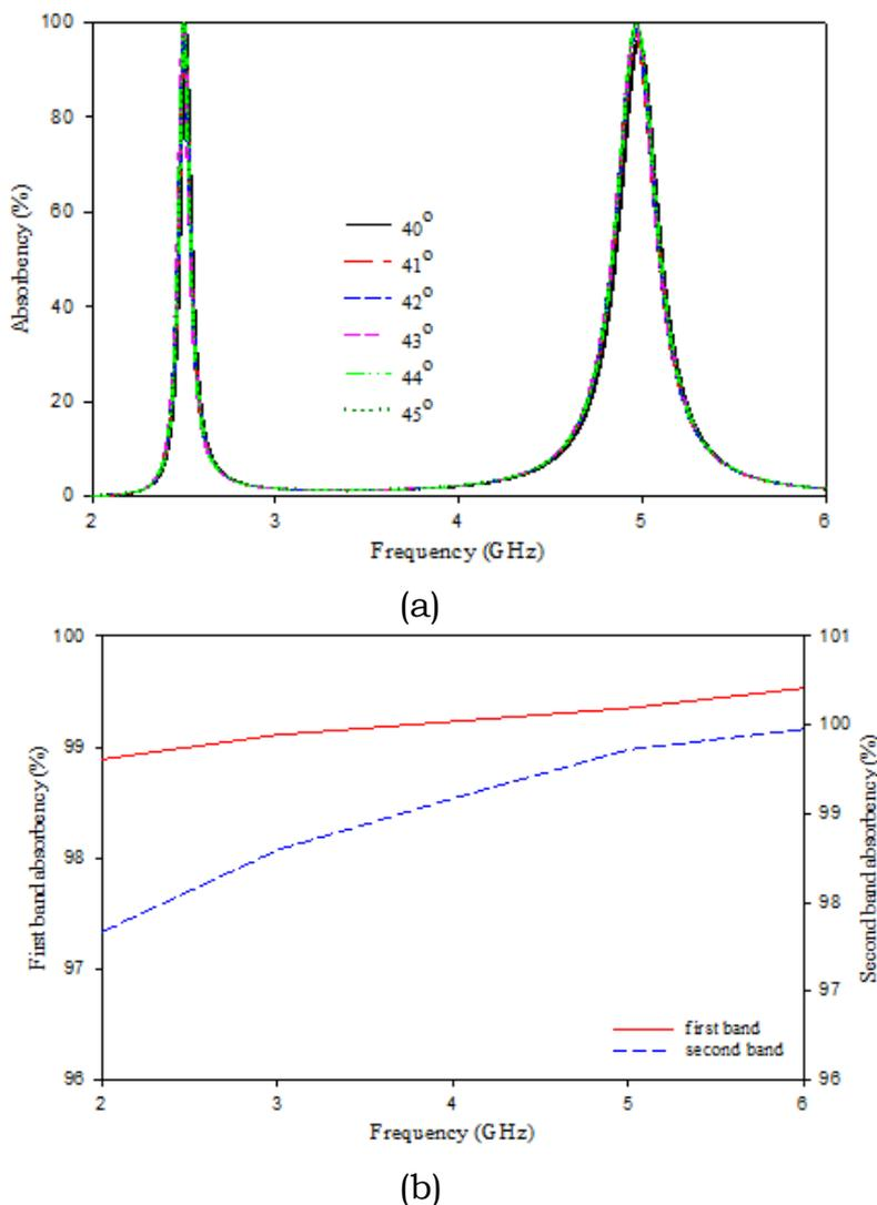
Figure 4: Simulated absorption spectra: (a) for rotation angles from  $40^\circ$  to  $45^\circ$  and (b) at  $45^\circ$  for first band and second band
