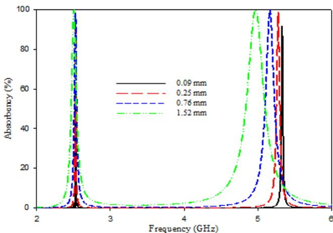
Figure 5: Dual band metamaterial absorber based on simulated absorption spectra according to the dielectric thickness
