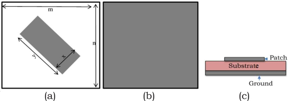
Figure 1: The views of dual band metamaterial absorber: (a) front; (b) back; and (c) side.
