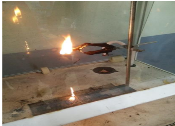
Figure 7: Horizontal flameability test
