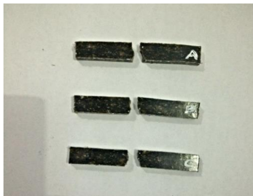
Figure 7: Charpy impact test on specimen
