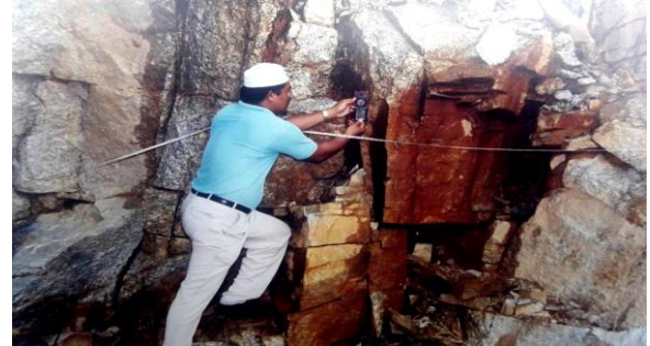
Picture 4: Geology Compass Instrument is used to measure the angle of dip and the slope direction of fracture
