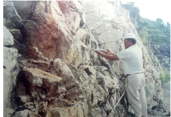
Picture 6: Schmidt Hammer Equipment used to measure the uniaxial compressive strength on fracture wall
