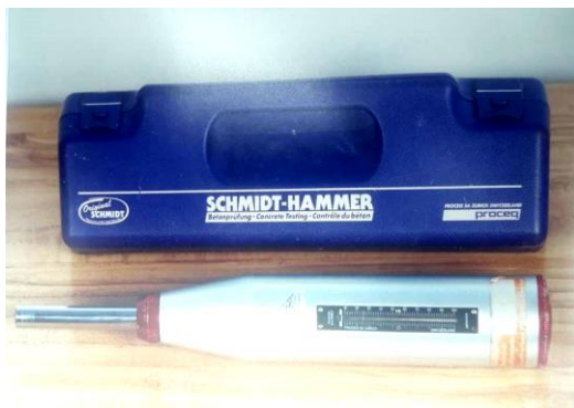
Picture 7: Schmidt Hammer Equipment is used to measure the uniaxial compressive strength of the fracture wall
