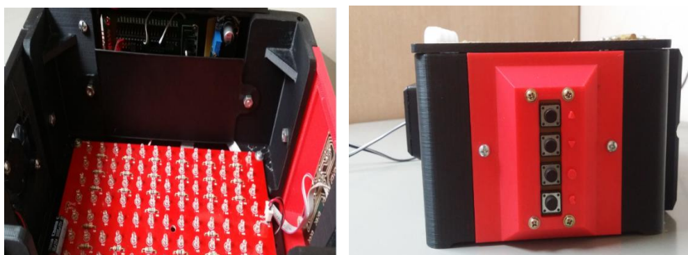
(a) Inside of the casing showing the UV LED assembly and controller circuit
