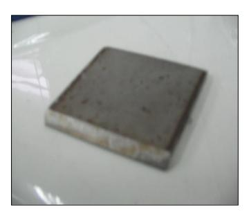
Figure 4: Stainless Steel 316L (sheet)
