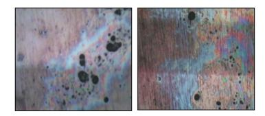
Figure 9: Effect HCl to corrosion in a surface of specimens
