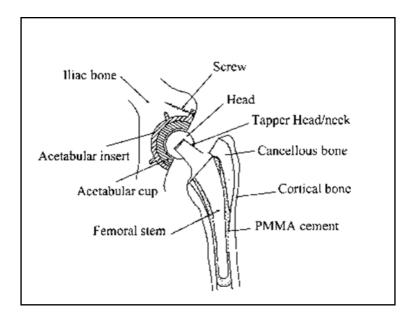
Figure 1: Total hip joint prosthesis components (L. Duisabeau, 2004)
