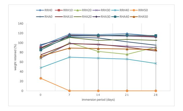
Figure 5: The weight of RRH-concrete and RHA-concrete after subjection in acid sulphuric solution
