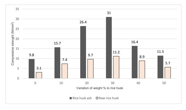
Figure 2: Variation of 28 days compressive strength for different mixture proportion
