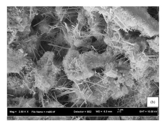
**Figure 4:** The bonding of C-S-H in Reco-block characterized by FESEM in (b) 2.50kX magnification
