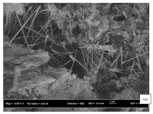
**Figure 4:** The bonding of C-S-H in Reco-block characterized by FESEM in (a) 5.00kX
