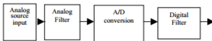
Figure 1. The data acquisition system signal chain can utilize analog or digital filtering techniques or combination of both
