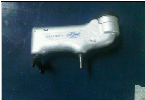
Rajah 6: Alat Pengujian Kekerasan ( Barcol Hardness - Colwa )
