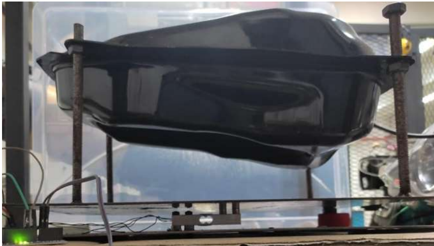
Figure 2: Electronic fuel weight scale setup
