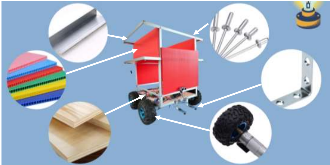
Figure 5: Materials used to construct the IAR casing
