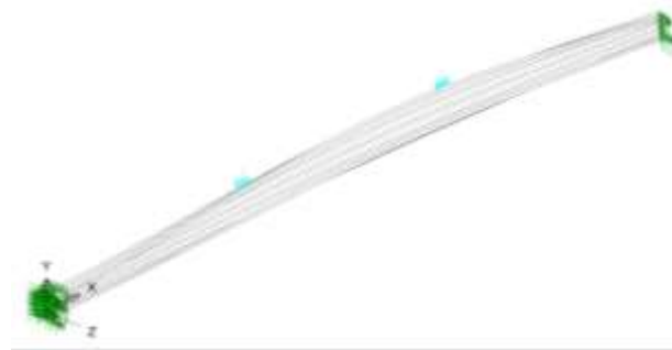
Figure 5: Failure mode of pinned-roller-lipped channel beam without concrete infill
