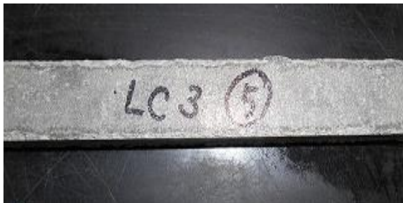
Figure 3: Cement composites with the addition of 17.5 wt. % quarry dust
