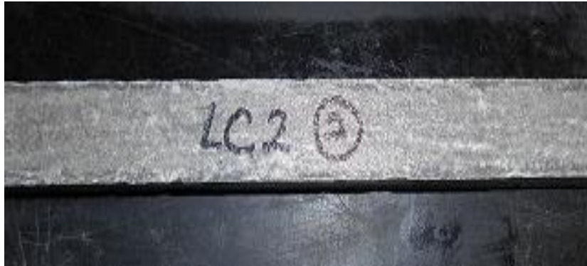
Figure 2: Cement composites with the addition of 12.5 wt. % quarry dust
