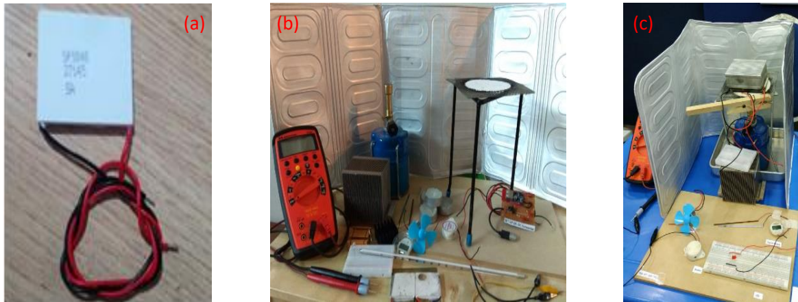
Figure 2: (a) TEG module, (b) Experiment Setup, (c) Open-Circuit with measurement and application test
